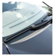
Reinstall the wiper arm protective cover.
