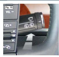
For rear window wiping (which is intermittent only), push the control lever towards the instrument panel one detent (Fig. 10).
