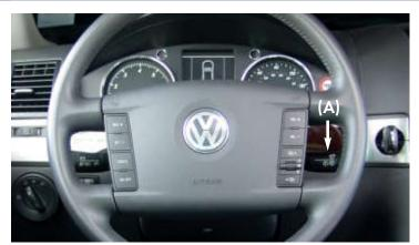
The windshield wiper control lever (A) operates both the windshield wipers and the windshield, rear window, and headlight washer systems.
