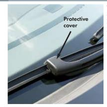
To change a wiper blade, you must first remove the protective cover from the windshield wiper arm mechanism.
