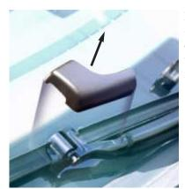
Remove the protective cover by lifting up at the edges, and pulling it upward (set it aside for reinstallation).
