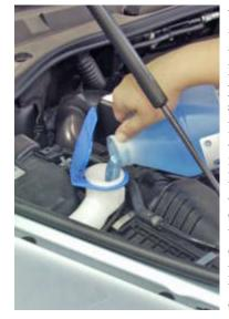
Your Touareg has been factory filled with a premium windshield washer solvent. For daily commuters, refill your windshield washer system with a premium pre-mix solution to remove accumulated airborne dirt, road grime, and road salts. For intensive cleaning, such as daily commutes near construction sites, or in areas with extreme airborne dust, dirt or pollutants, mix a premium concentrate with water to accommodate daily cleaning conditions.
