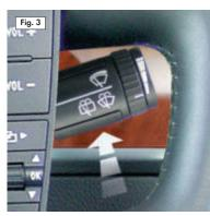
For continuous high speed windshield wiping, only the control lever needs to be utilized (Fig. 3).
