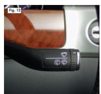
To turn off all wiper functions, push the control lever to a horizontal position and turn off the rear wiper (Fig. 12).
