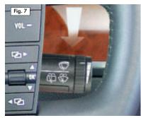
To quickly wipe the windshield with a brief wipe, push the control lever down and release it (Fig. 7).
